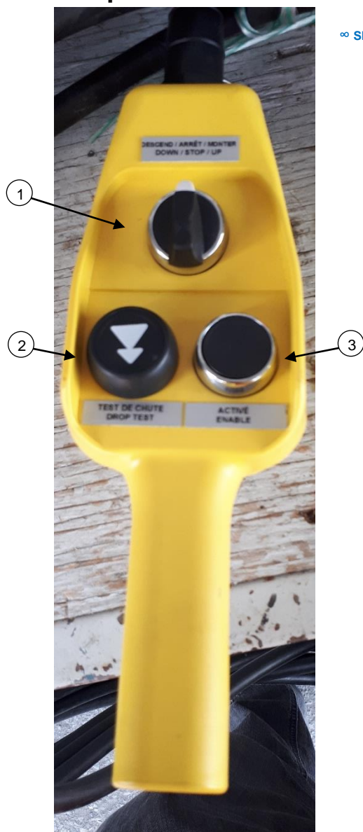
Figure 27 – Drop test remote control
